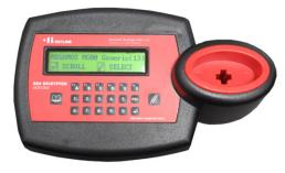
Use the arrow button to scroll through different chip types. Once you have desired chip type press the WRITE button to confirm.
