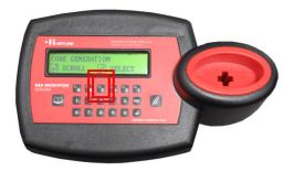
Press the F3 function to access the Code Generation screen.
