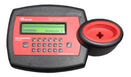
Code can now be manually entered (if known) using the keypad or for a random value select the arrow button, then press WRITE button.
