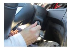
Use the TKM/GKM key to turn the vehicle's ignition to the ON position for 5 seconds, then OFF for 2 seconds, then remove the key. Repeat this step for a total of 8 times.
