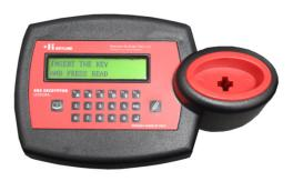
When prompted, insert the original key into the reader and press READ.
