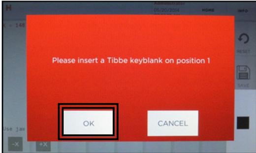
Insert a standard Tibbe key blank in jaw at **position 1** as shown in pictures
