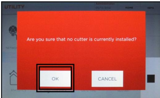
Confirm cutter removal, select **OK**. Jaw will move into position.
