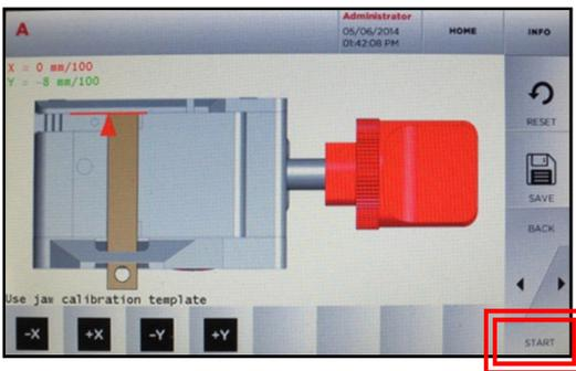
Install Jaw to far left of carriage until it stops. **CLAMP TIGHT WITH JAW LEVER.**
