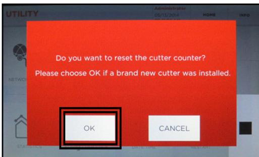
Select **OK** to reset cutter counter (only if cutter is brand new)
