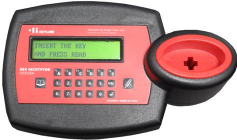
When prompted, insert the original key into the reader and press READ button.
