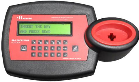
When prompted, insert the original key into the reader and press READ button.
