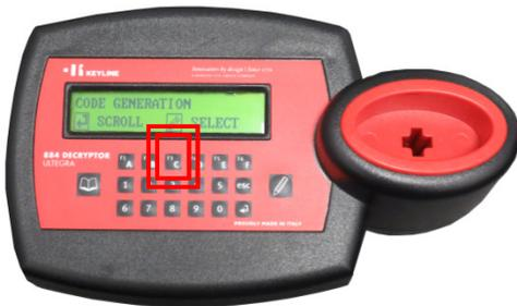
Press the F3 function to access the Code Generation screen.
