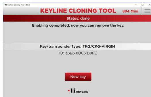
Enabling process completes. Once prompted, remove the TKG head; it can now be used as a key
