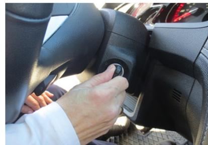
Use the TK100/GK100 key to turn the vehicle's ignition to the ON position for 5 seconds, then OFF for 2 seconds, then remove the key. Repeat this step 4 more times.
