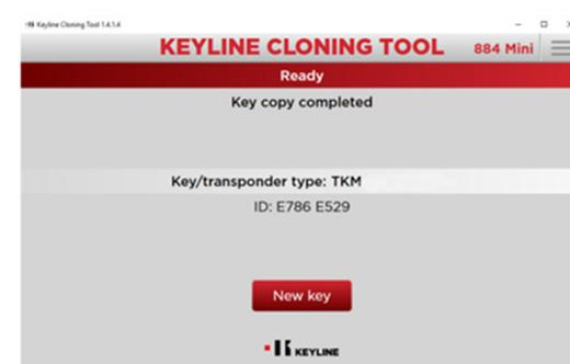
Key copy is complete; take the new TKM/GKM key to the vehicle and confirm vehicle starts.
