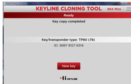
When 'Key copy completed' displays, key is complete
