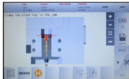
Insert Tibbe key in 0 position. Select CUT
