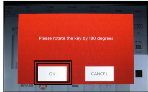
Rotate key for second side cutting, Select **OK**
