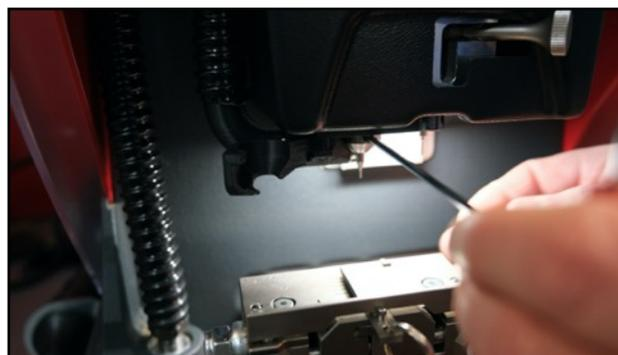
**REMOVE CALIBRATION TRACER T00 from the cutter spindle. PRESS OK**
