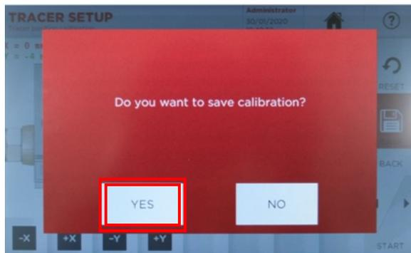
Write down the X & Y values and **PRESS THE SAVE BUTTON**. **PRESS YES** to save the results.
