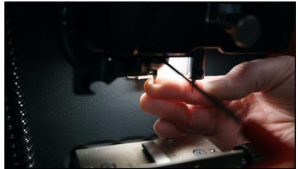
Install the T00 Calibration **TRACER** from the tool kit into the cutter spindle. Tighten the set screw and **CLOSE THE SHIELD**. PRESS OK
