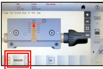
To change the material type, simply touch the BRASS icon on the screen until you reach the desired material; **BRASS**, **STEEL**, **NiSi** (Nickel Silver) or **ALU** (aluminum)
