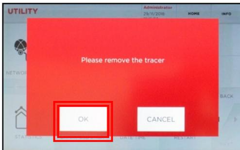
Remove tracer using 2.5mm allen tool, then select **OK**
