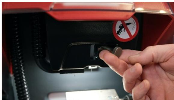
When prompted, loosen the tracer knob, **LIFT THE TRACER KNOB** and **MOVE IT TO THE RIGHT**. Close the shield. **PRESS OK**
