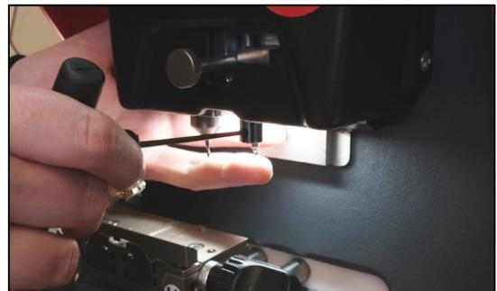
Install new tracer until it stops and tighten down set screw with 2.5mm allen tool
