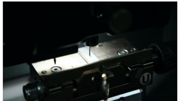
Loosen the tracer knob, lower the **TRACER** until it lands on the setup template, **tighten** the **KNOB**. PRESS **OK**
