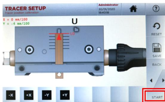
Insert setup template into jaw
