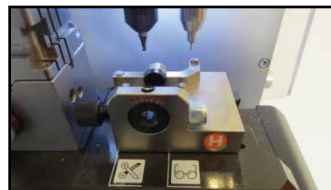
Move jaw to cutting position, close shield and select OK
