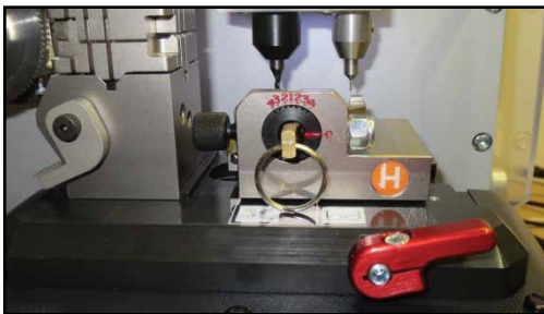
Fig. 2 Template turned to 0 position. Tighten with left thumb wheel
