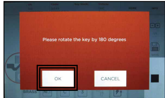
Flip key in jaw, removing key shavings with brush, select OK
