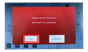
Loosen the tracer knob, lower the TRACER and tighten the knob. PRESS OK
