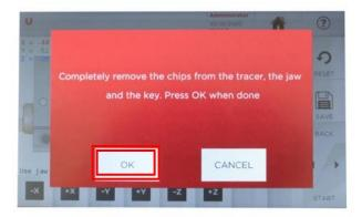
Completely remove the **CHIPS** from the **TRACER**, the **JAW** and the **KEY**. **PRESS OK**.
