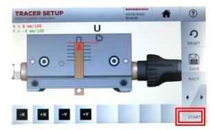
Insert the calibration template as shown. **PRESS START**.
