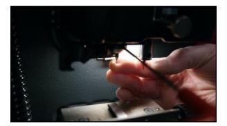
Install the T00 Calibration **TRACER** into the cutter spindle. Tighten the set screw and **CLOSE THE SHIELD**. **PRESS OK**
