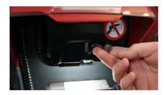
When prompted, loosen the tracer knob, LIFT THE TRACER and MOVE IT TO THE RIGHT. Close the shield. PRESS OK
