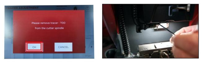
REMOVE CALIBRATION TRACER T00 from the cutter spindle. PRESS OK
