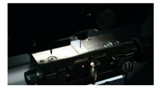
Loosen the tracer knob, lower the TRACER, tighten the KNOB. PRESS OK
