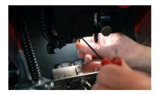
REMOVE the V037 CUTTER. PRESS OK
