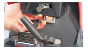
Install new tracer until it stops and tighten down set screw with 2.5mm allen tool You must perform the tracer setup, tracer adjustment and jaw calibration
