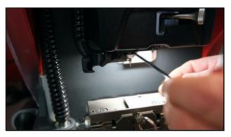
**REMOVE CALIBRATION TRACER** T00 from the cutter spindle. **PRESS OK**
