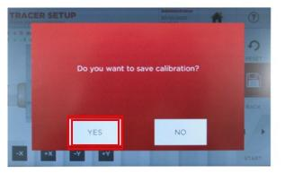
Write down the X & Y values and **PRESS THE SAVE BUTTON**. **PRESS YES** to save the results. **PRESS THE BACK BUTTON** after checking their values (see next page).
