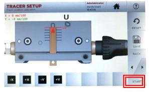
Insert the calibration template as shown. **PRESS START**.
