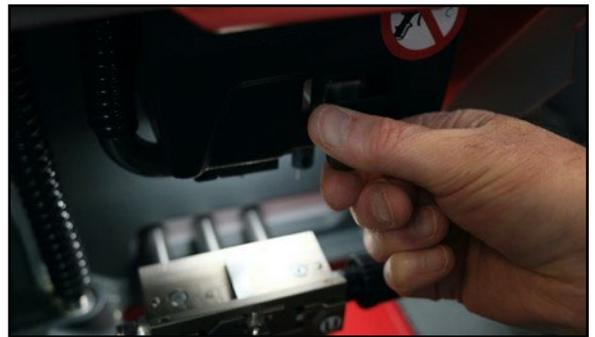
Loosen the tracer knob, lower the **TRACER** and tighten the knob. **PRESS OK**
