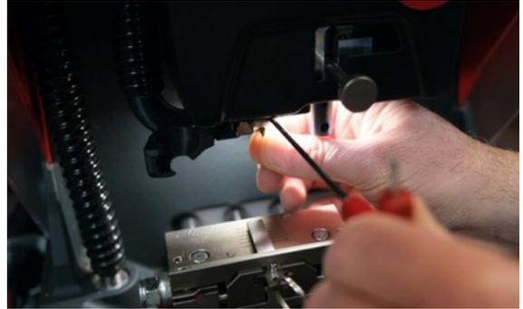
REMOVE the V037 CUTTER. PRESS OK
