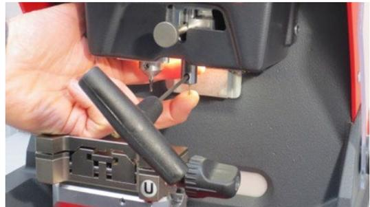
Install new tracer until it stops and tighten down set screw with 2.5mm allen tool
