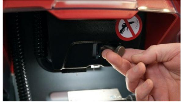
When prompted, loosen the tracer knob, **LIFT THE TRACER** and **MOVE IT TO THE RIGHT**. Close the shield. **PRESS OK**
