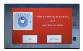
Follow the machine prompts for each cut position until the first side of key is complete. After cuts are complete, **machine will prompt to put key into position 1** (i.e. home position so key can be removed), then select **OK**.
