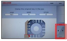
Insert key on jaw, then **remove tip stop**. **Close shield** and select **NEXT**
