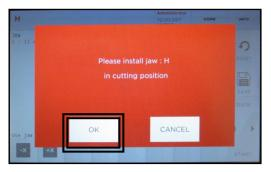
Install jaw H in cutting position, select **OK**
