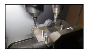
Install cutter until it drops down and rests on top cutter landing dot (shown at left). Tighten cutter set screw.
