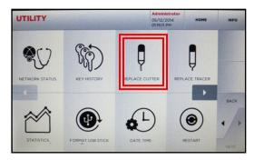
Select **REPLACE CUTTER**, make sure appropriate jaw is installed
