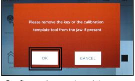
Confirm no keys or templates are installed on jaw, select **OK**
