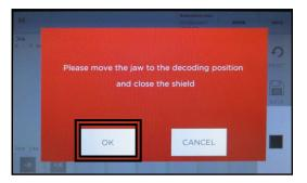
Move jaw to DECODING position, select **OK**
