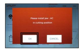
Install Jaw AC in cutting position, select **OK**. Utility screen appears, select **HOME** to go to Main Menu.
