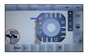
Once key cutting is complete, put additional duplicate key to be cut into jaw and select **CUT**.
