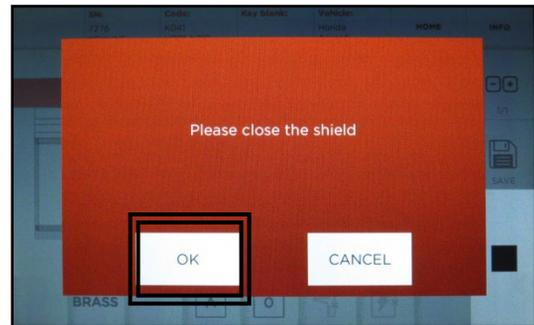
Close the shield and select **OK**. Jaw moves into position
