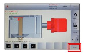
Install Jaw to far left of carriage until it stops. <u>CLAMP TIGHT WITH JAW</u> LEVER.
