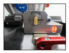
**Turn template to position 0** (as shown in above picture) and tighten left side thumb wheel to lock in position. Select **OK** and jaw calibration will begin.
