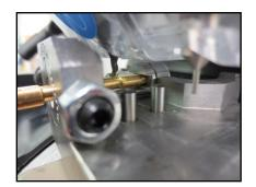
Install cutter until it drops down and rests on top of the Tibbe key blank. Tighten cutter set screw. Jaw will move into position after selecting **OK**.
