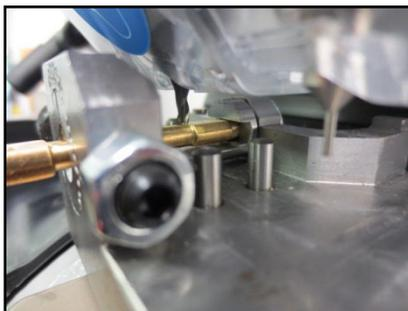
Install cutter until it drops down and rests on top of the Tibbe key blank. Tighten cutter set screw. Jaw will move into position after selecting **OK**.
