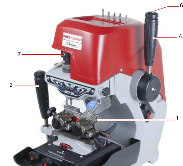
3. Then, use the lever (2) to move the carriage under the cutter-tracer point unit (3).
