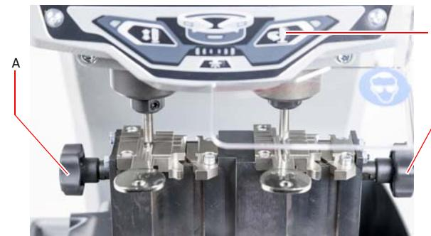
**Note:** Cisa keys that cannot be placed in the standard socket on the left grip can be locked on the right-side grip on a dedicated holder that prevents them from tilting.
