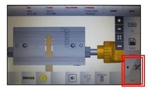
Insert key into jaw as far as possible but not past the back of the jaw. Hold key flat in jaw while tightening. Select CUT
