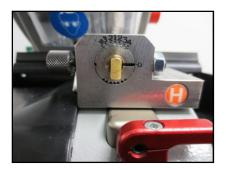
**Turn template to position 0** (as shown in above picture) and tighten left side thumb wheel to lock in position. Select **OK** and jaw calibration will begin.
