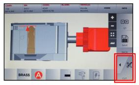
Insert key correctly on jaw, paying close attention to the stop position for the key blade, then select **CUT**
