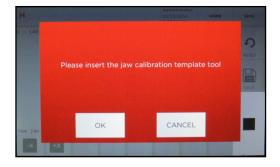
Insert Tibbe jaw calibration template (metal Tibbe template included with H Jaw). Insert template completely into jaw. Tighten front set screw with included Allen wrench.
