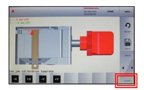
Install Jaw to far left of carriage until it stops. <u>CLAMP TIGHT WITH JAW LEVER.</u>
