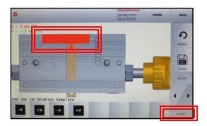
Install Jaw to far left of carriage until it stops. CLAMP TIGHT WITH JAW LEVER.
