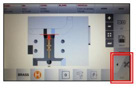
Insert Tibbe key blank on jaw in position 0, select **CUT**
