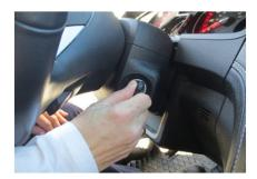
Use the TKM/GKM key to turn the vehicle's ignition to the ON position for 5 seconds, then OFF for 2 seconds, then remove the key. Repeat this step for a total of 4 times.
